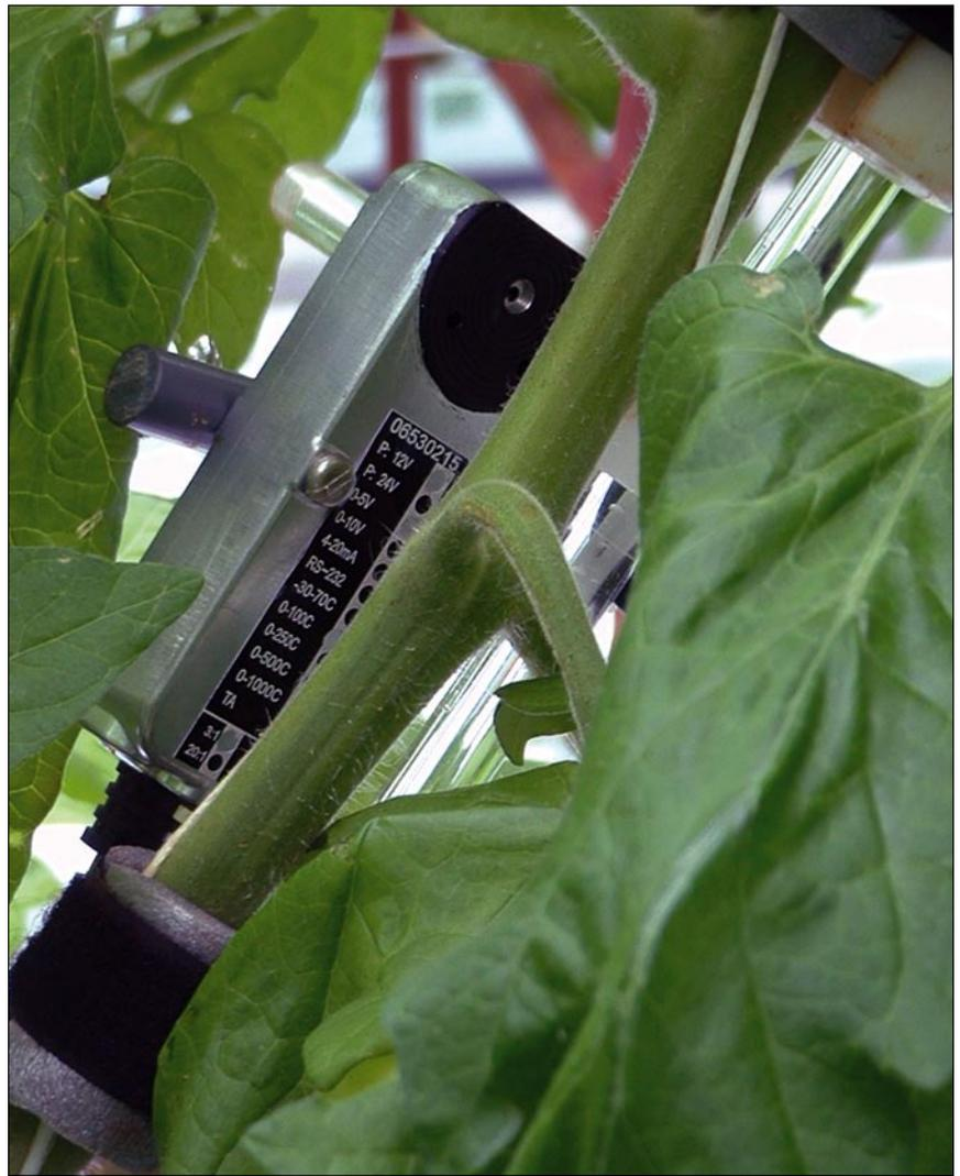
5 Infra-red sensor used to measure plant or plant organ temperature
