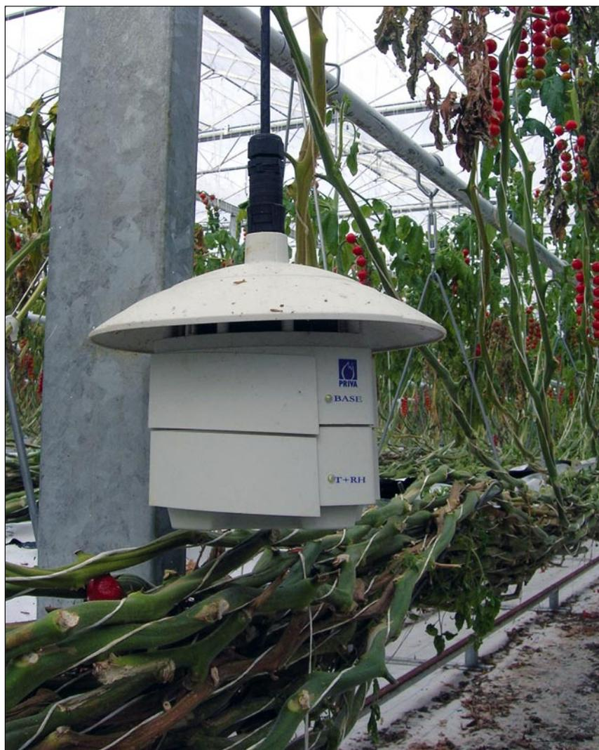
4 Measuring box incorporating an electronic humidity sensor
