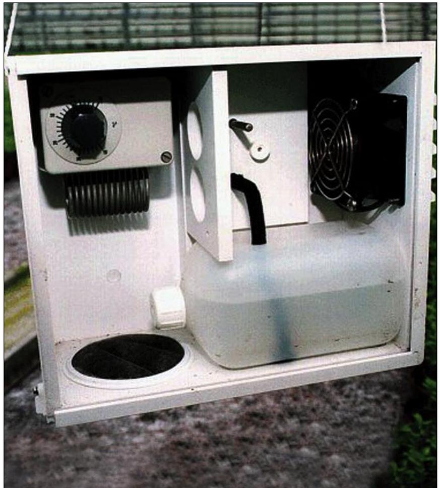
**3 Conventional measuring box design with ‘wet’ and ‘dry bulb’ sensors**
